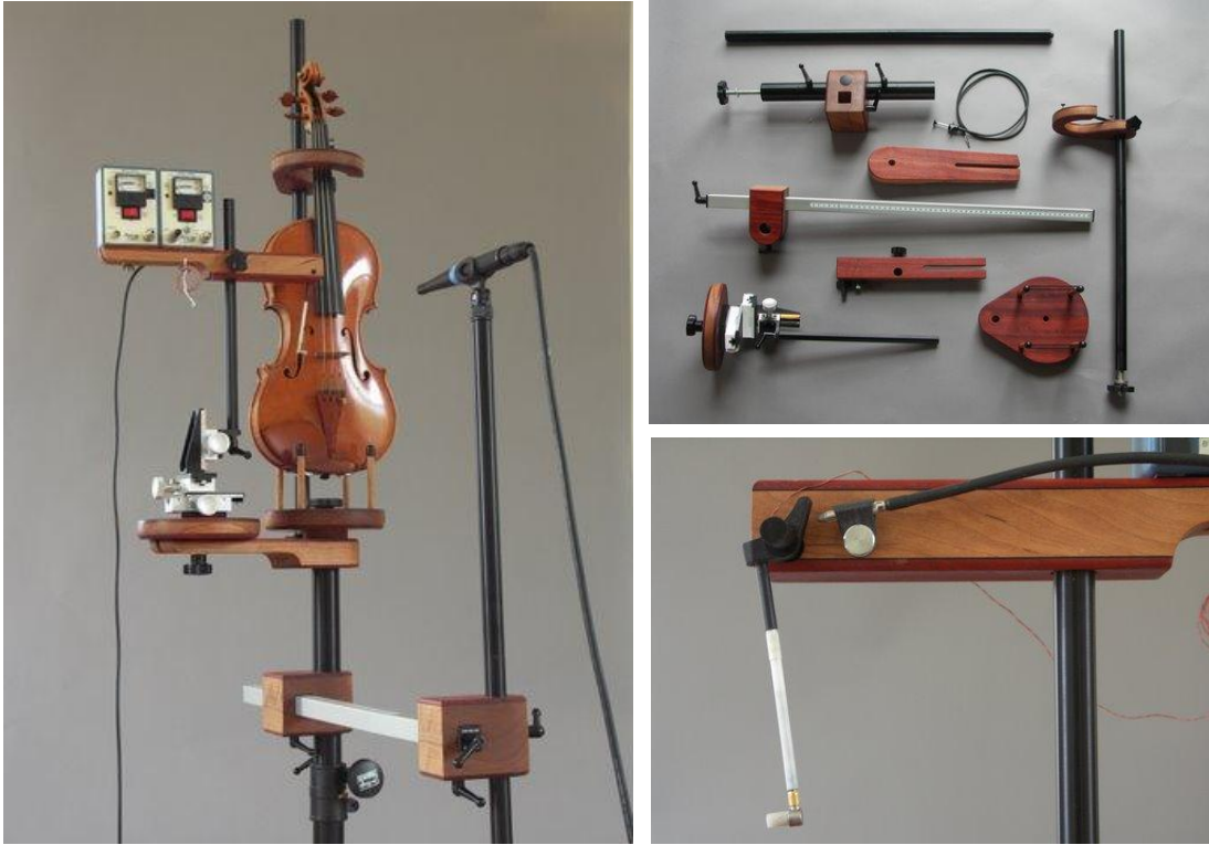
The Sound Radiation Rig – a tool for measuring the sound radiation of violins and violas. For further information, see www.josephcurtinstudios.com .
